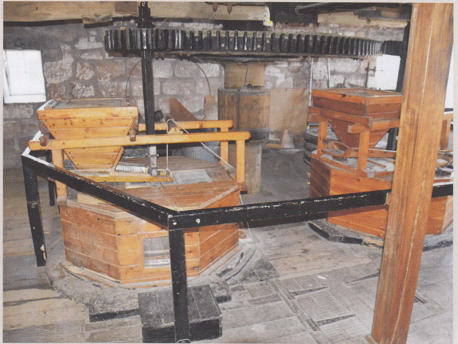
Grain was poured into the hopper on the first, or Stone Floor, from the top floor. The hoppers at Brindley's Mill are quarter scale replacements to help with a demonstration.
