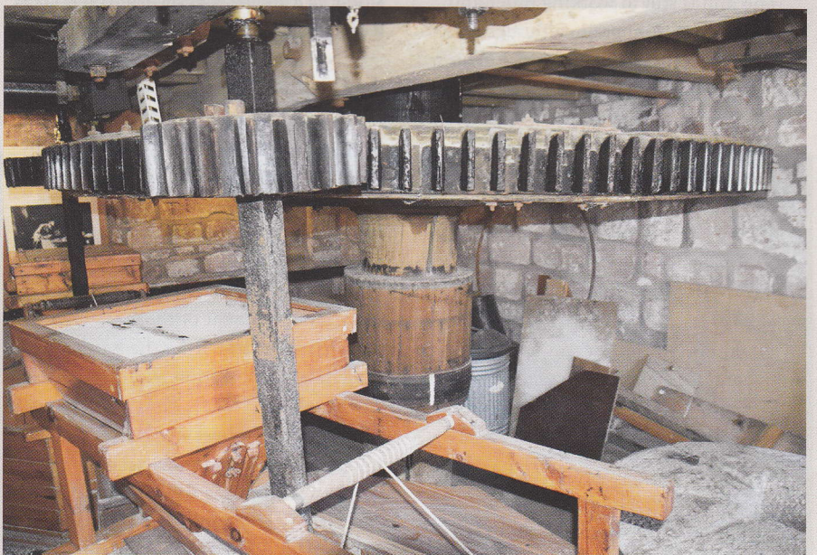
... and is then passed through the stone nut to the top runner stone.
