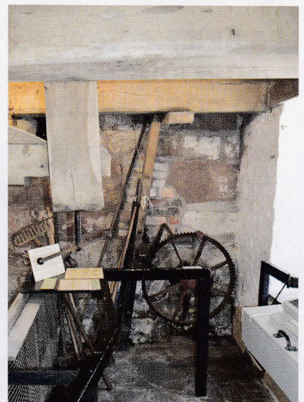
The geared wheel next to the window raises the sluice gate outside the mill. This allows the water to pass underneath to start the waterwheel, which is connected to the pit wheel by the axle tree.
