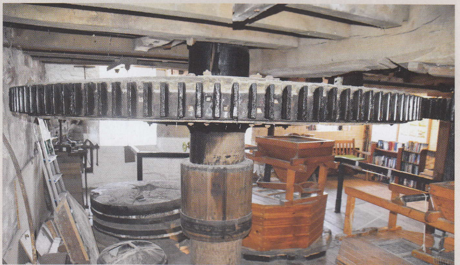
Power is taken from the vertical main shaft by the great spur wheel...
